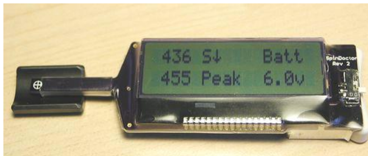
Measuring the concave surface of a motor magnet.
