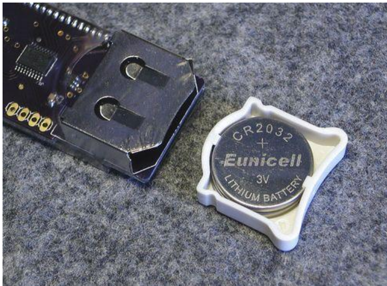
Battery Tray Removed
